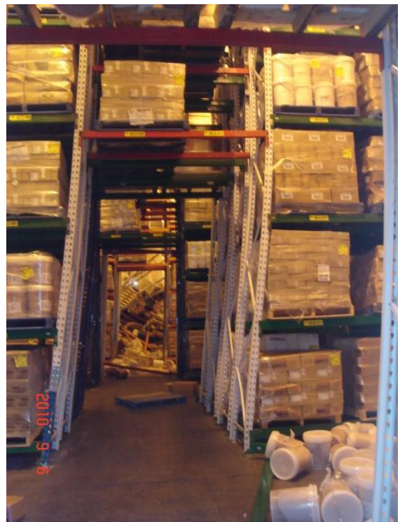
No.12 Double deep selective racking.
