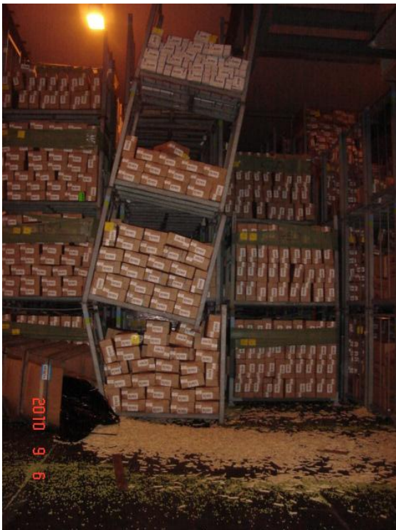
No.11 Distorted post pallets.
